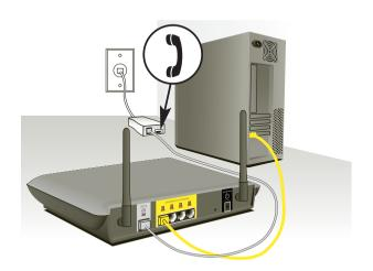
**Note:** One RJ11 telephone cord is supplied. When inserting an RJ11 plug, be sure the tab on the plug clicks into position to ensure that it is properly seated.
